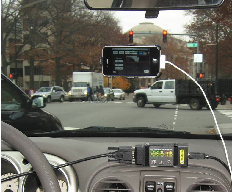
Figure 4.3: SignalGuru-enabled iPhone mounted on the windshield. The OBD-LINK device used to measure fuel consumption is also shown.
