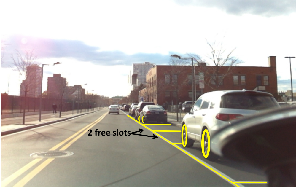
Figure 4.24: Parking service enabled by windshield-mounted smartphones and their cameras. The detected vehicle wheels and parking spot lines are shown with yellow ovals and lines, respectively. Two free spots are detected.
